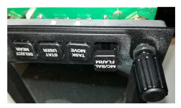
4. Select new o-ring and place it over the button axis (button should remain partialy in the housing !!!). Slide The rubber o-ring over the axis and push the button back in the housing. Adjust the o-ring height to a desired one, the button should be able to be pressed whitout sticking.
