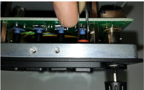
5. When satisfied whit the result, screw the housing back and test the buttons for functionality and press feeling.
