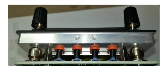
3. Using fine twezzers, partialy prime the desired button out of housing in fashion to remove the defected o-ring from the button axis.
